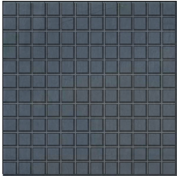
Fig.9: County grade 7mm thick Cwt-y-Bugail Dark Blue Grey slate slab, 300mm square, cut into nominal 25mm square mosaic 'tiles'.
